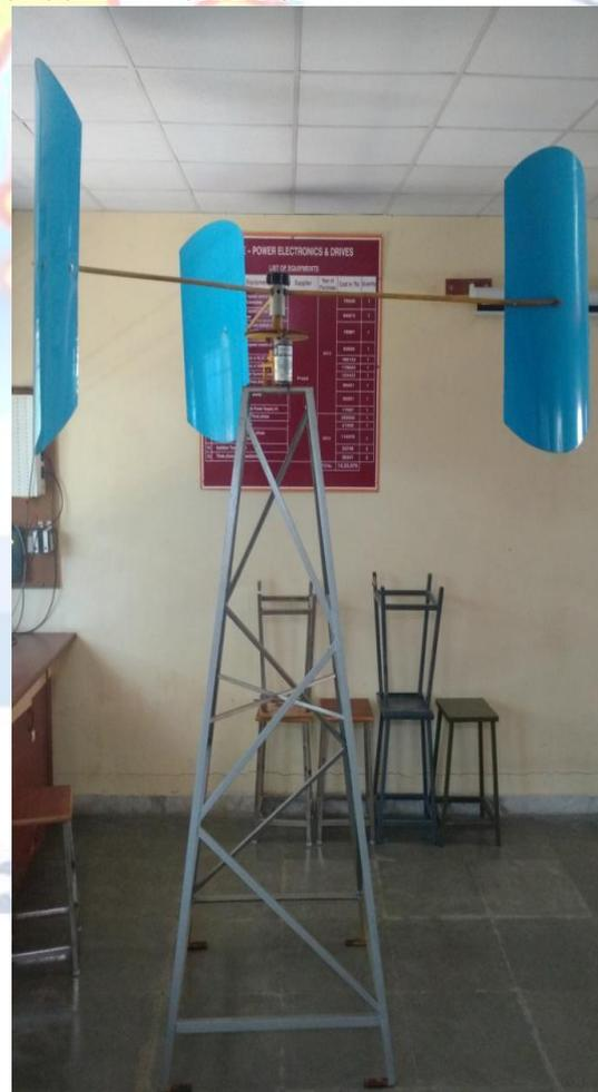
**BLADE:** In VAWT, the blades are made up of Aluminium sheet. It consists of 3 blades in parabolic shape.
