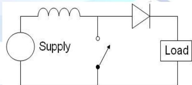
Figure Boost Converter Schematics
