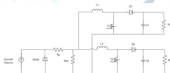
Figure Circuit diagram of SIDO Boost converter
