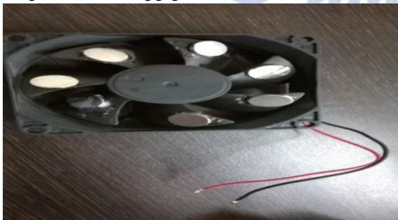
Fig. 2 Fixing magnets on motor blades
