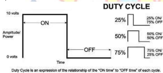
Pulse Width Modulation, or PWM, is a technique for getting analog results with digital means. Digital control is used to create a square wave, a signal switched between on and off. This on-off pattern can simulate voltages in between full on (5 Volts) and off (0 Volts) by changing the portion of the time the signal spends on versus the time that the signal spends off. The duration of "on time" is called the pulse width modulation.
