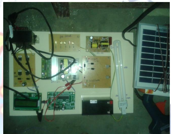
Fig.6.Photo of PV inverter
