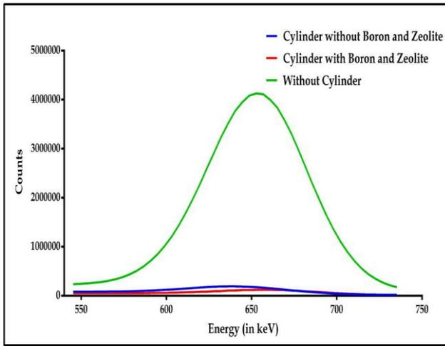
**Fig.1 Comparison Between Concretes and Without Concrete Gamma Radiation Absorption**
