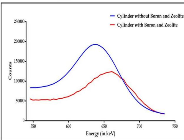
**Fig.2 Comparison Between Concretes Gamma Radiation Absorption**
