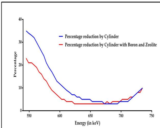
**Fig.3 Percentage Reduction of Cesium (137Cs) Gamma Energy by cylinder with and without Boron and Zeolite**
