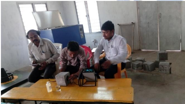
Fig 1 UPV cube testing
