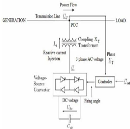
Fig 4: basic block diagram for static compensator
