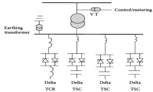
Fig 5: Thyristor Switched Capacitor
