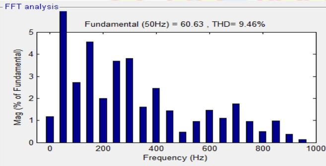
Fig 8: FFT analysis for Source current.
