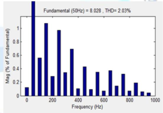
Fig 12: FFT analysis for Source current.
