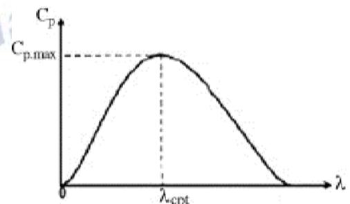
Fig 3: Power coefficient Vs Tip Speed Ratio
