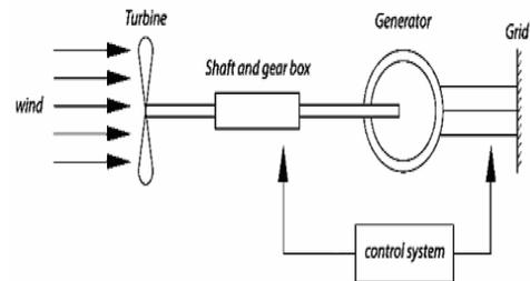
Fig.2 basic schematic diagram of wind turbine
