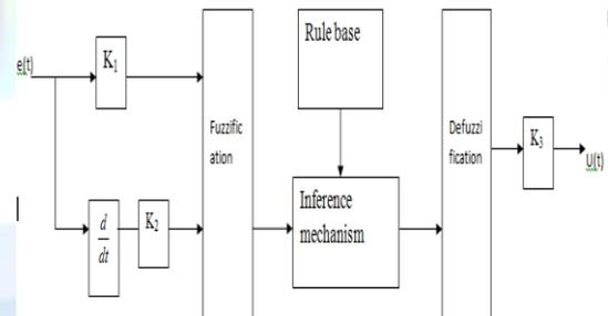
Fig.6 Fuzzy Logic Controller block diagram
