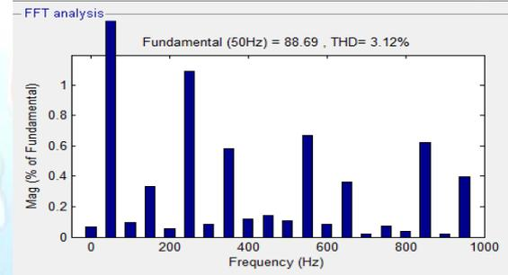
Fig 11: FFT analysis for Source current.
