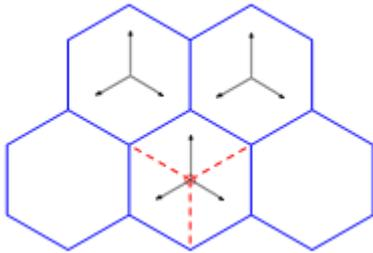
**Figure 2: Rhombus cells created by replacing the omni directional antenna at the center of a hexagon by three directional antennas.**
