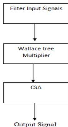
Fig:2 Flow of FIR Design
