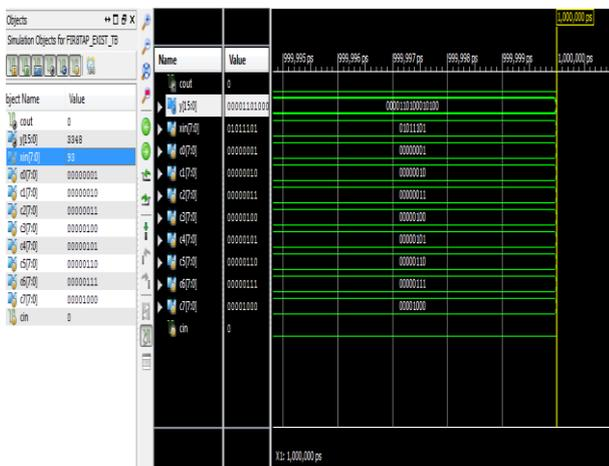
**Fig:13 Waveform for FIR Filter**
