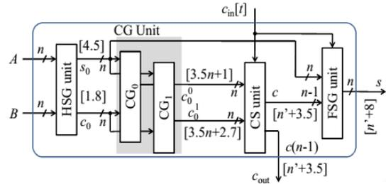
Fig:3 New Carry select adder design
