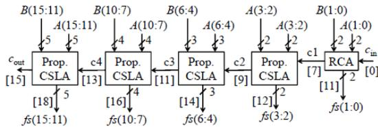
**Fig:9 16 Bit Carry select adder Design**
