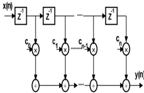
Fig:1 FIR Filter Design
