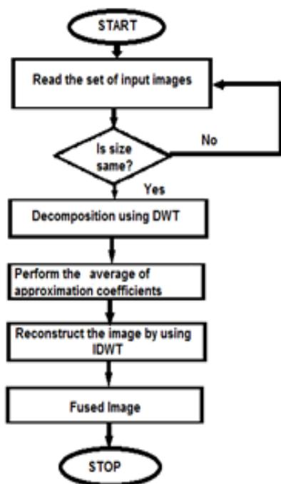
Fig 1.Flow chart of image fusion process
