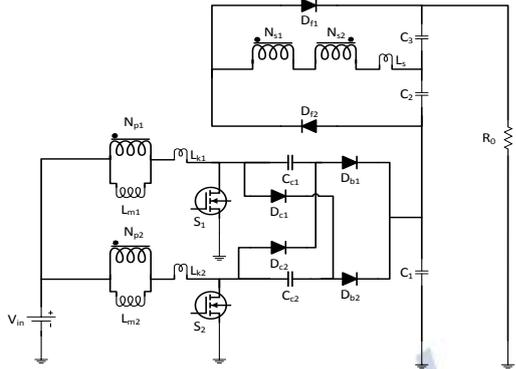
Fig. 3. Equivalent circuit of proposed converter
