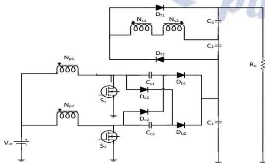
Fig. 2. Proposed high gain converter
