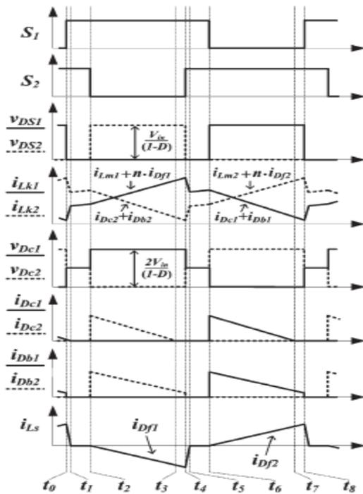
Fig. 4. Steady waveforms of proposed converter
