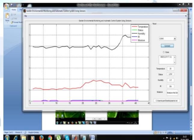
**Fig 5 variation in temperature, soil moisture and humidity with the time and are captured using MATLAB simulator**
