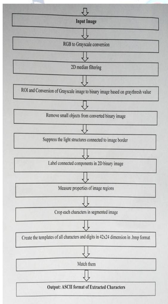
Figure 2:- Flowchart diagram of proposed system
