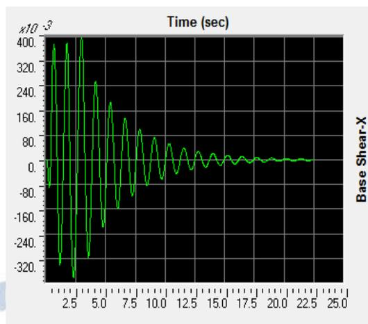
Fig 10:- Base Shear-Time history of building with isolator
