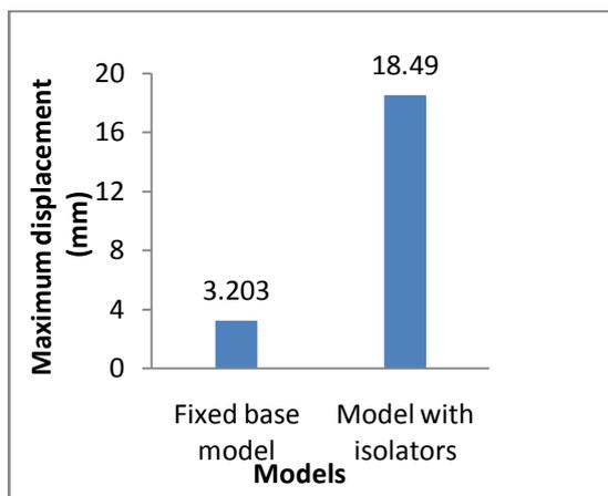
Fig 7:- Maximum Displacement for both models
