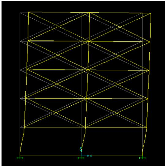
**Fig3 :- Deformed shape of fixed base model**
