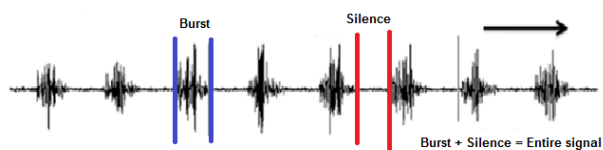
Fig.2: Representation of silence part in a signal
