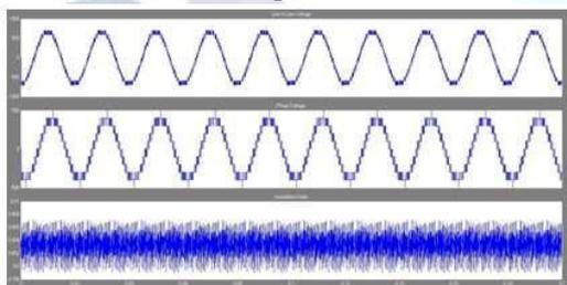
Figure 9: Line Voltage and Phase Voltage with Modulation Index Equal to 0.7
