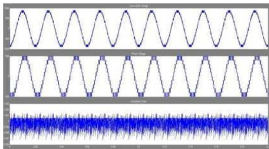
Figure 7: Line Voltage and Phase Voltage with Modulation Index Equal to 0.9
