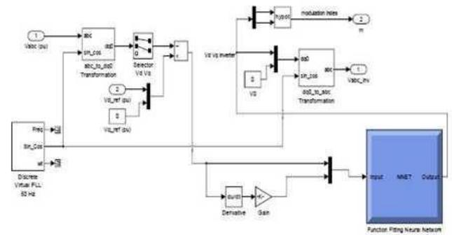
Figure 5: Artificial Neural Network Applied to 11 Level Cascaded H Bridge Multi Level Inverter
