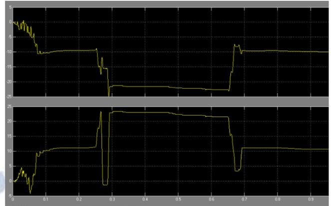
**Fig 6: Active and reactive power provided by the shunt-connected multifunctional converter to compensate the voltage sag of 0.15 Pu.**
