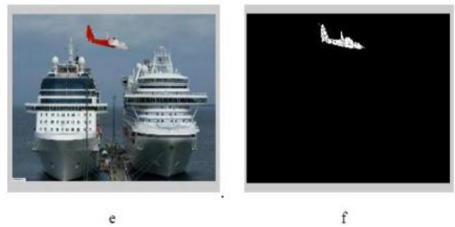
Fig. 6.(a) Original harbor ships, (b) original aero plane, (c) watermarked harbor ship image, (d) watermarked aero plane image, (e) tampered harbor ship image, (f) detected tampered region
