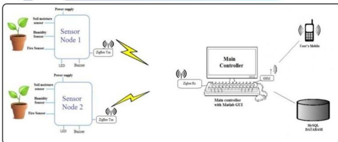
Figure 1: Architecture of Automated Irrigation System
