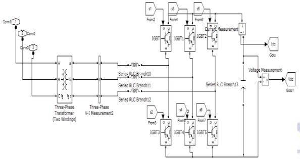
Fig 4.1 Control scheme of STATCOM
