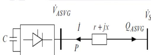
Fig 3.1 basic model of STATCOM
