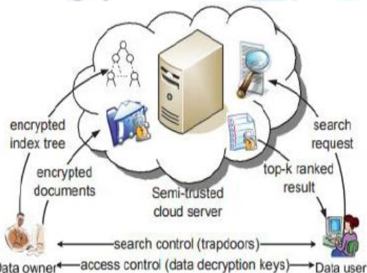
Fig. 1. The architecture of ranked search over encrypted cloud data
