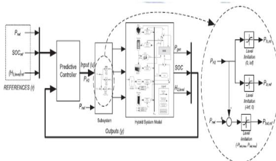
Fig.2. Overall scheme of the energy dispatching based on MPC.
